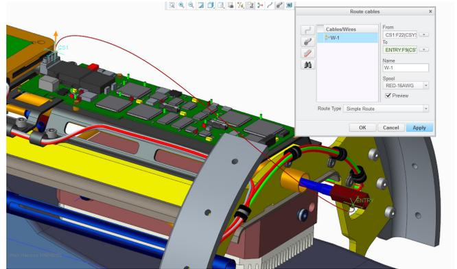
Determine the connections either manually or from logical information. PTC Creo PCX automatically generates a simple path which then enables the user to find the optimum path faster.
